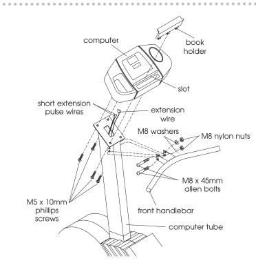
Figure 8- Install Front Handlebar and Computer
